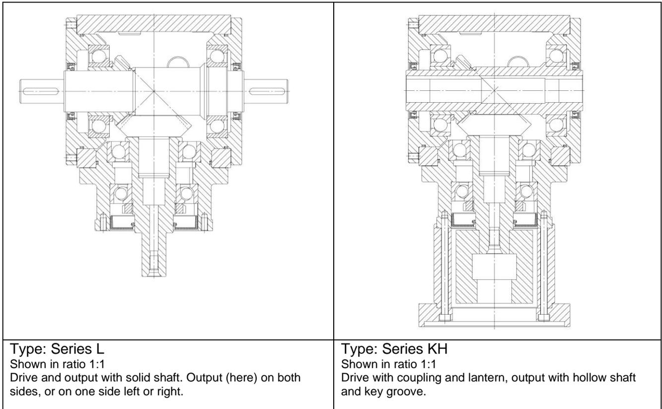
Shaft bearings with angular contact ball bearings, lubrication with synthetic gear oil ISO VG 150
