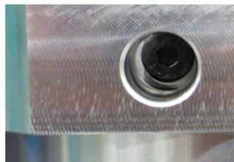
Tighten the tensioning screw in the clamping hub with a suitable  $M_A$ ,
